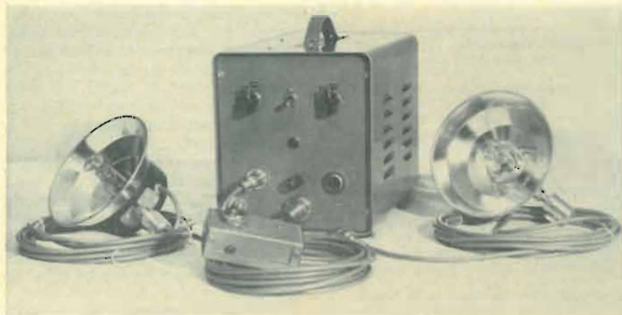
The complete slave assembly consists of two flash lamps, the remote trigger unit, and the power supply/timer. Cables may be any convenient length, depending on your needs.
