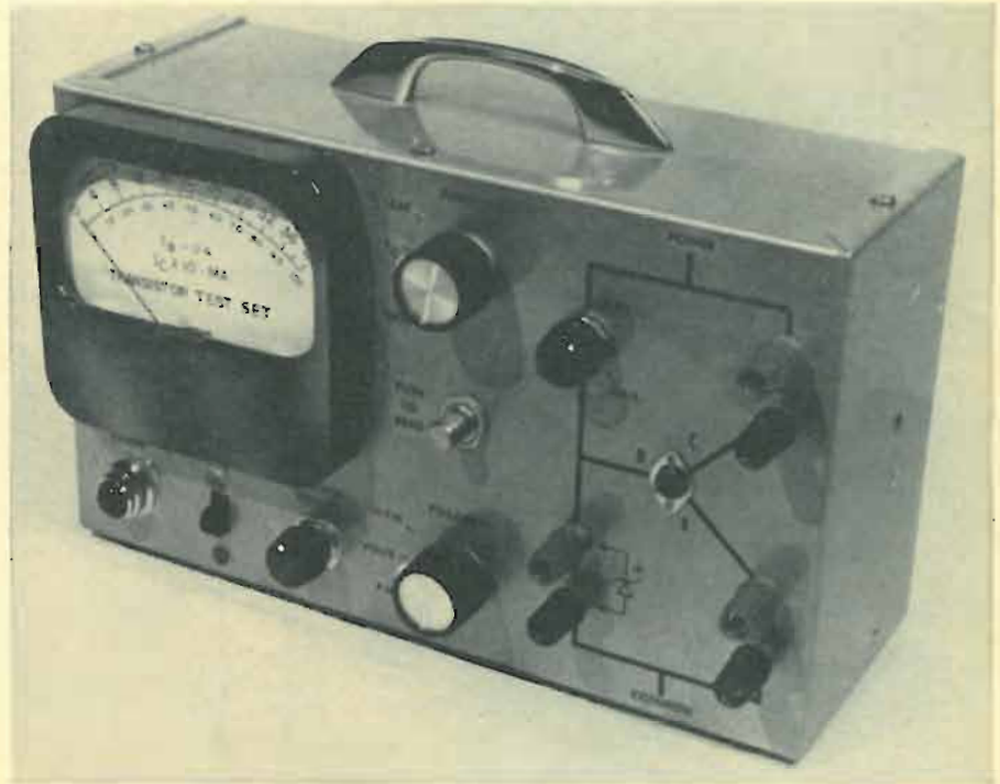
The black tape lines on front panel make it easy to connect semiconductors for test.
